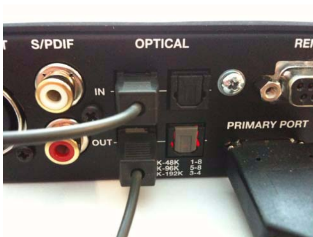
Figure 1. Optical loop back connections
