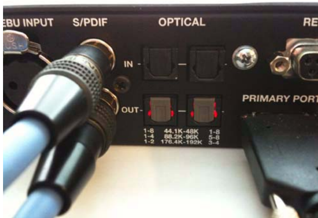
Figure 10. Coaxial (S/PDIF) loop back connections
