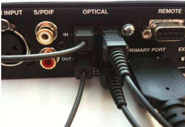
Figure 4. Optical loop back connections
